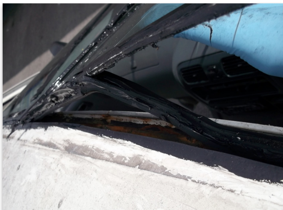
No adhesion between windscreen aperture due to non use of primer and poor fitting
