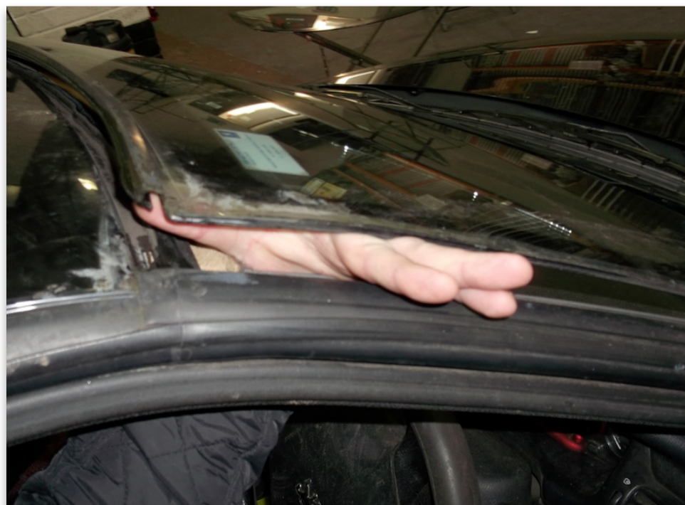
No adhesion between windscreen and aperture
