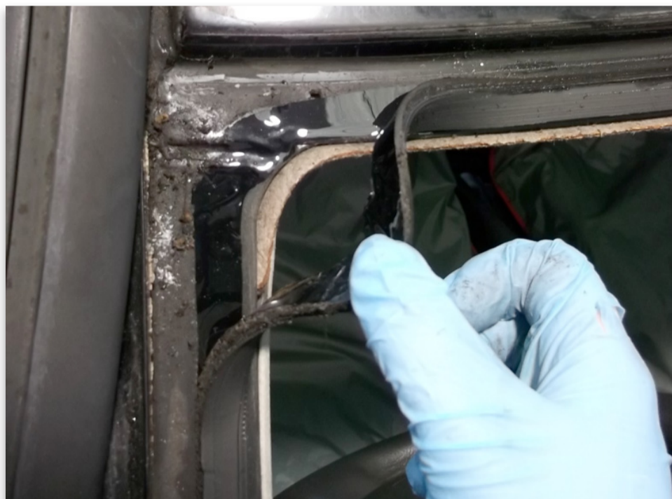
No adhesion between aperture and bond/glue
