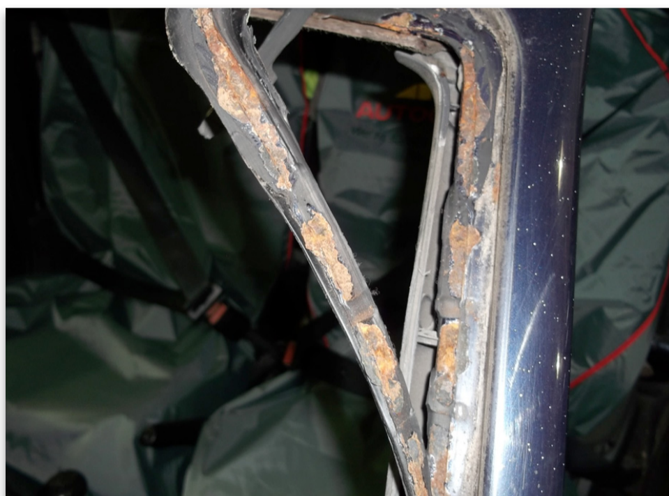
Corrosion due to lack of primer causing damage to the aperture
