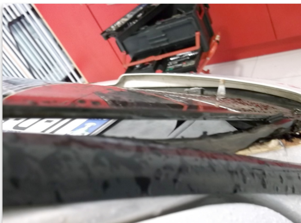
No adhesion between windscreen and aperture caused by lack of primer and incorrect fitting procedures
