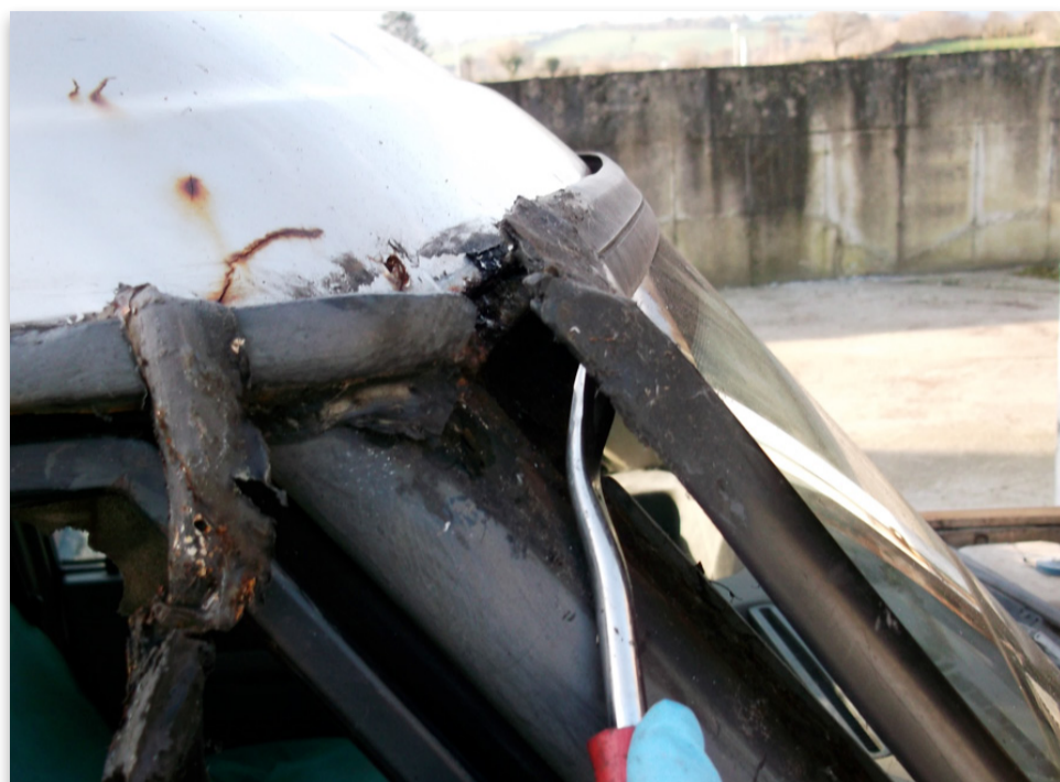
No adhesion between windscreen and aperture and severe damage caused by corrosion
